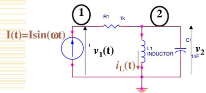
$$\begin{aligned} \frac{1}{R_1} v_1(t) - \frac{1}{R_1} v_2(t) &= i(t) \\ -\frac{1}{R_1} v_1(t) + \frac{1}{R_1} v_2(t) + i_L(t) + C_1 \frac{\partial v_2(t)}{\partial t} &= 0 \\ v_2(t) - L \frac{\partial i_L(t)}{\partial t} &= 0 \end{aligned}$$
