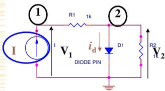
$$\begin{aligned} \frac{V_1 - V_2}{R_1} &= I \\ \frac{V_2 - V_1}{R_1} + i_d(V_2) + \frac{V_2}{R_2} &= 0 \\ i_d(V_2) &= I_s (e^{\frac{V_2}{V_T}} - 1) \end{aligned}$$
