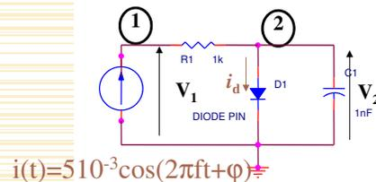
$$\frac{1}{R_1} v_1(t) - \frac{1}{R_1} v_2(t) = i(t)$$
