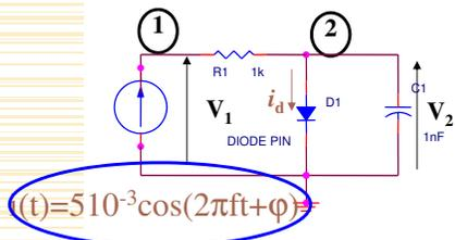
$$\frac{v_1(t) - v_2(t)}{R_1} = i(t)$$
