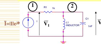
$$\frac{1}{R_1} \bar{V}_1 - \frac{1}{R_1} \bar{V}_2 = \bar{I}$$
