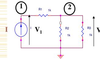
$$\frac{1}{R_1} V_1 - \frac{1}{R_1} V_2 = I$$
