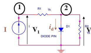
$$\begin{aligned} \frac{1}{R_1} V_1 - \frac{1}{R_1} V_2 &= I \\ -\frac{1}{R_1} V_1 + \left( \frac{1}{R_1} + \frac{1}{R_2} \right) V_2 + I_s (e^{\frac{V_2}{V_T}} - 1) &= 0 \end{aligned}$$
