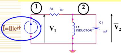
$$\frac{\bar{V}_1 - \bar{V}_2}{R_1} = \bar{I}$$
