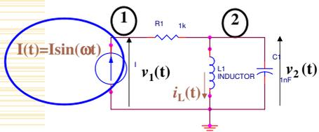
$$\begin{aligned} \frac{v_1(t) - v_2(t)}{R_1} &= i(t) \\ \frac{v_2(t) - v_1(t)}{R_1} + i_L(t) + C_1 \frac{\partial v_2(t)}{\partial t} &= 0 \\ v_2(t) - L \frac{\partial i_L(t)}{\partial t} &= 0 \end{aligned}$$
