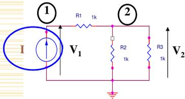
$$\frac{V_1 - V_2}{R_1} = I$$
